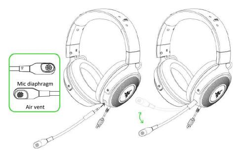
(1) Make sure the mic diaphragm is in front and the air vent is facing away from your mouth. The recommended mic-to-mouth distance for optimal sound capture is 1.5 cm to 3 cm (0.59 in to 1.18 in).
